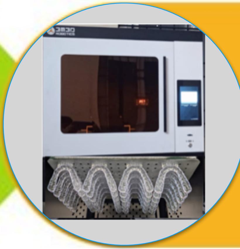
The created 3D model fed into the 3M3D slicer software and the aligners printed directly in 3M3D DigiDenture Printer using Memory shape Special resin.
